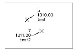
Point Label Style - Point#, Elevation, Description in a Dragged State with Stacked Text in the correct order.
