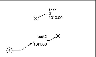
Problem 1: Point Labels have leader attached to the wrong side of the label when dragged to the left of the point.
