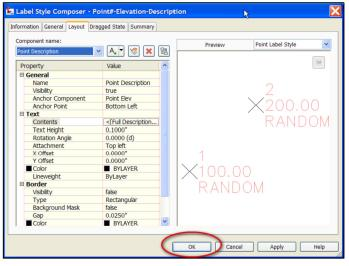
Finish the required changes to the Point Label Style. You should now be able to use this style in it's dragged state. You should now have the leader attached to the correct side of the text and the components in the correct order.
