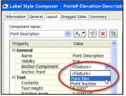
Getting the Point Description component lined up with the Elevation component is detailed in the screen captures to the left
